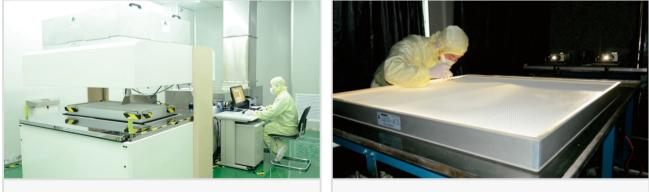
A-PLUS testing procedures for overall efficiency include laser particle counters with liquid or solid aerosol challenge.
